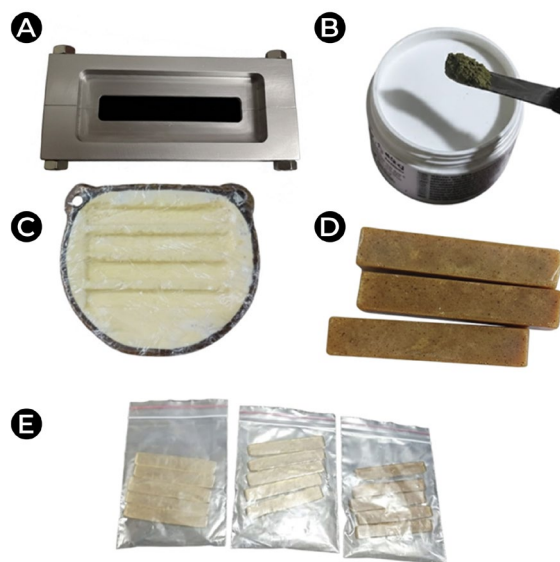
Fig. (1). Fabrication of Specimens (A) Stainless Steel Die (B) Alkali Treated Moringa Powder (C) Plaster Mould (D) Acrylic Bars for Testing (E) Prepared Samples Sealed in Pouches.
